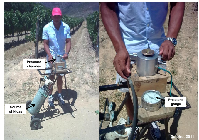
Figure 1. Example of a pressure chamber used to measure leaf water potential (photo from A. Deloire, South Africa).
