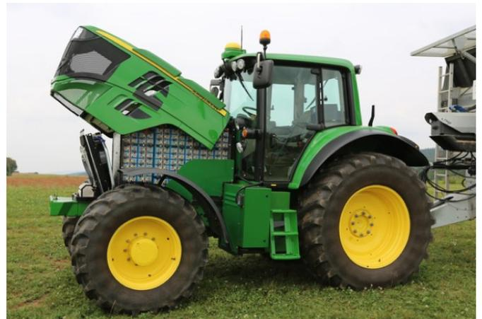
**Figure 1.** John Deere's battery electric tractor SESAM presents an enormous battery pack<sup>4</sup>.
