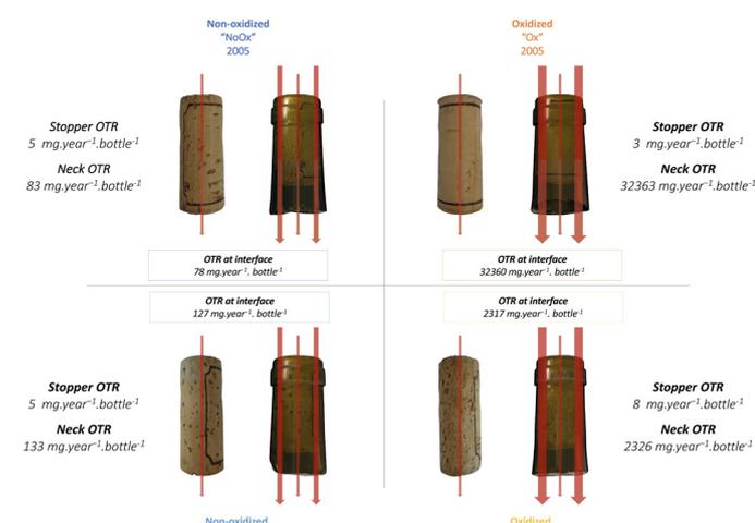
**Figure 2.** Oxygen transmission rate (OTR) measured through the cork stopper alone (cork), the stopper + neck assembly (neck) and the interface.
