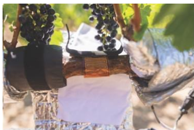
FIGURE 1. A dismantled installation of sensors for sap measurement with the heat balance method.
